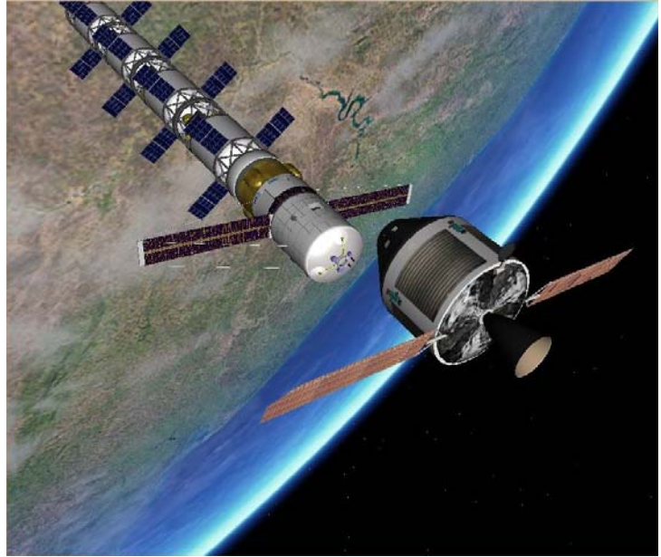
Figure 1. This Orbiter screen shot shows the Mars-ready “stack” of crew and propulsion modules that have been assembled in low Earth orbit, along with an approaching crew transfer vehicle (NASA CEV 2005 concept). In addition to its spaceflight modeling abilities, the quality of Orbiter’s 3D graphics makes it an excellent visualization tool.
